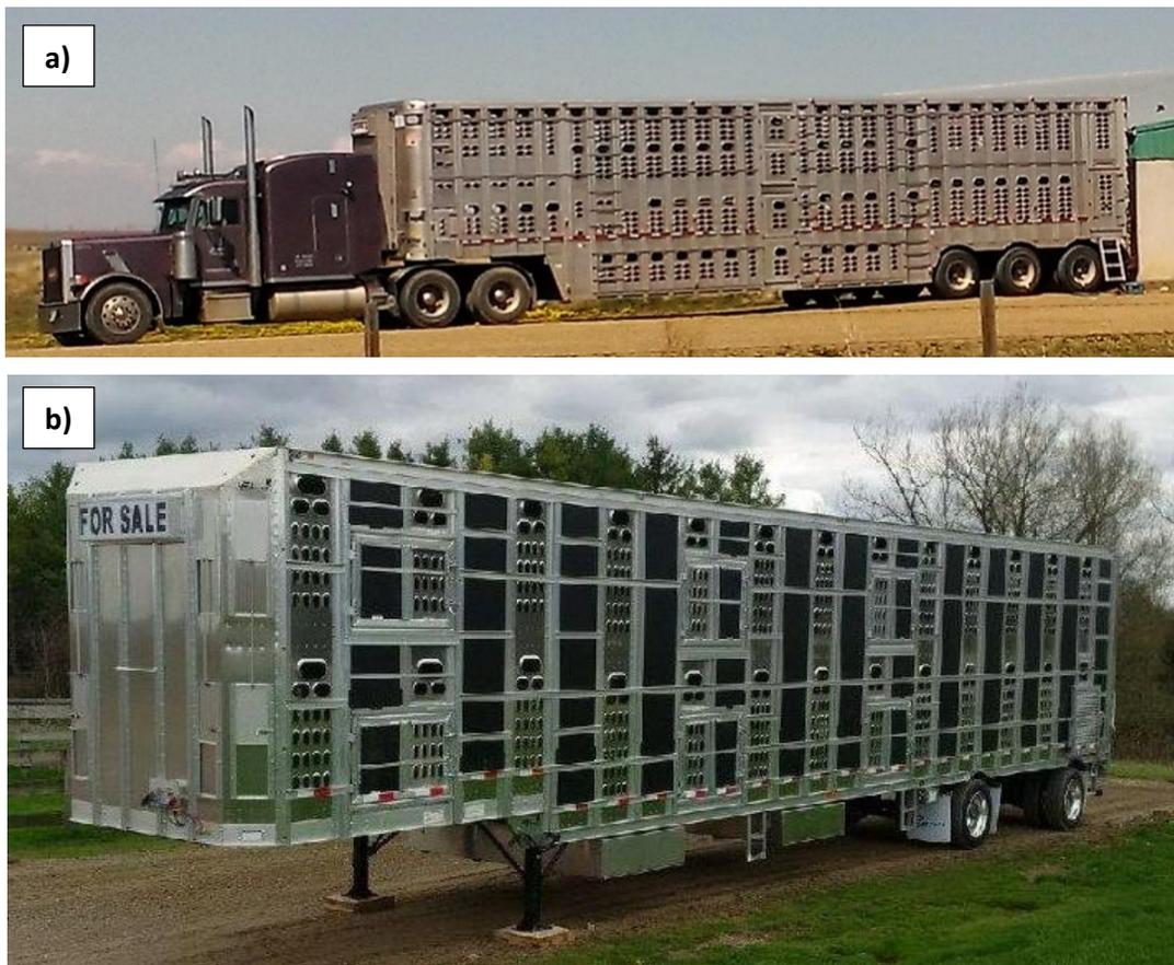
Figure 4: Types of vehicles used in Canada: a) “pot-belly”; and b) flat deck trailers. Courtesy of A. Hurst (Luckhart Transport, Sebringville, ON)
