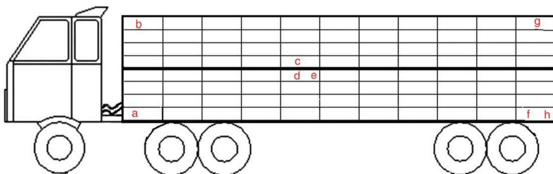
Figure 7: A diagrammatic representation of standard articulated lorry for poultry transport with 11 stacks 2 modules high. Each module contains 12 drawers (4 high x 3 wide). Labels a-h mark logger positions. At logger positions a-g, loggers were located in the central drawer, locations e and h on the side of and outer drawer of a module (Richards et al., 2012).
