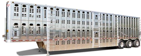
Figure 5: Tri-Axle “Pot-Belly” Trailer (Source: Wilson Trailer Company)
