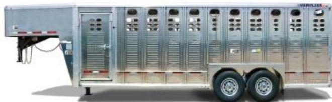
Figure 3: Tandem Axle Gooseneck Stock Trailer (for use with pickup truck) (Source: Wilson Trailer Company)
