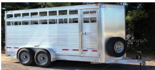
Figure 2: Tandem Axle Bumper-Pull Stock Trailer (Source: Eby Inc.)
