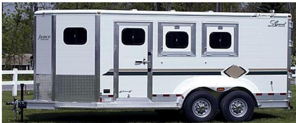
Figure 7: Bumper Pull (Ball and Socket) Horse Trailer (Source: Jamco Trailers)
